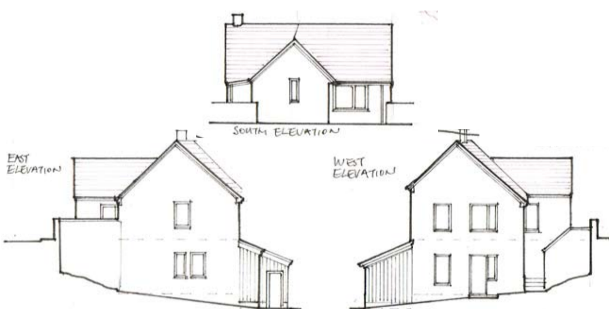
Home No.2: A four-bedroom home addressing Pike Lane with a modest facade of render and clay tile, extending down to its gardens below
