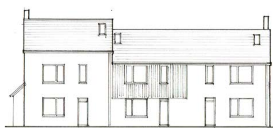
Homes Nos.4 to 8: A row of three- and four-bed attached houses forming a street frontage, clad in render and larch with slate and zinc roofs
