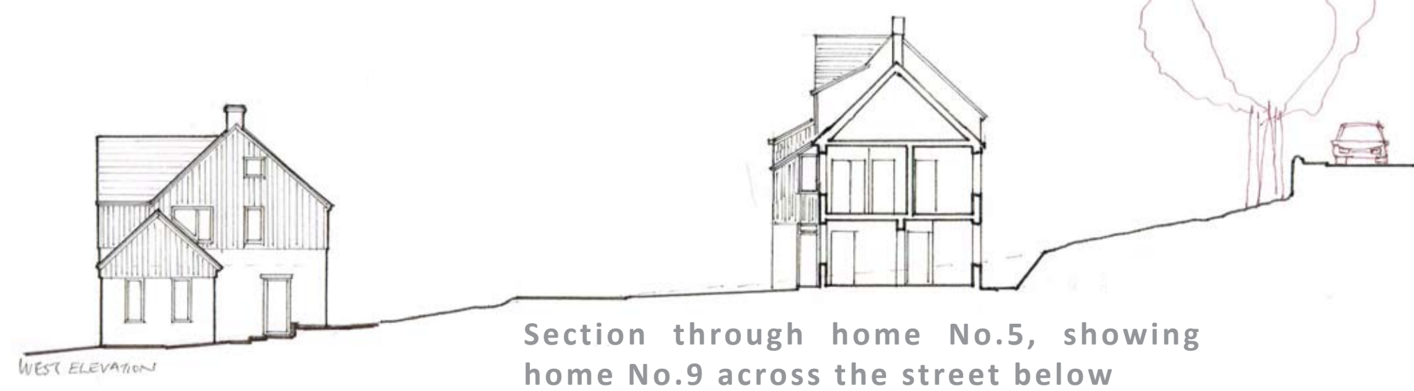
Homes Nos.4 to 8: A row of three- and four-bed attached houses forming a street frontage, clad in render and larch with slate and zinc roofs
